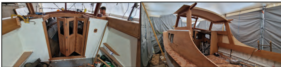
Building and fitting companion way doors, structural components: wheelhouse and main bulkhead
