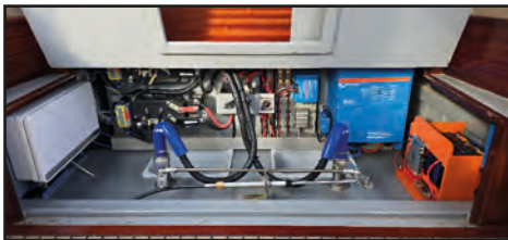
Motor controllers, power distribution, and wiring for switch panel - both shown incomplete
