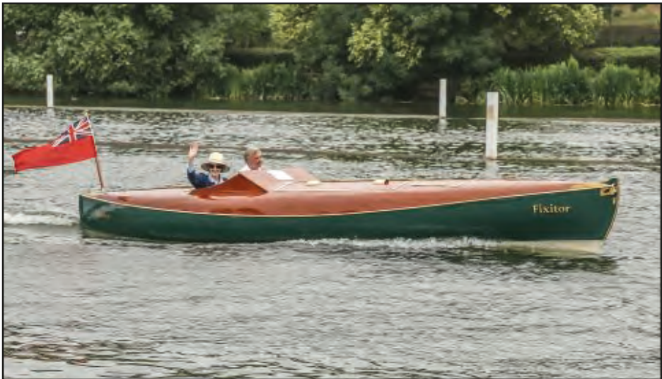
Example of a turtle foredeck on 'Fixitor' c1900 builder unknown.
