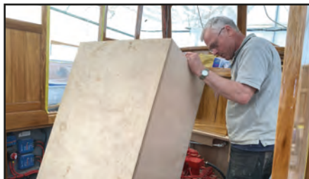
Making the engine box for DLS Deenar
