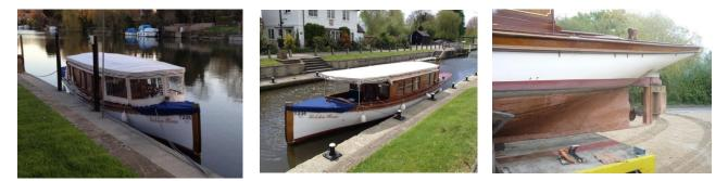
Built c1885 - all wood double planked teak and oak hull, of carvel construction with caulked seams. Originally steam powered, she was converted to diesel in the 1970's. History uncertain prior to 1974, when she was found abandoned in Goole and carefully restored over
